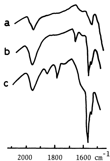
Fig. 3. IR spectra of PVC (a), and \text{H}_2 -absorbed [\text{4-Fe}]^{2-} (b) and \text{H}_2 -absorbed [\text{Mo-Fe}]^{3-} in the PVC matrices.
